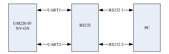
Figure 4-4 Connect COM to PC
