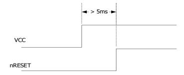
Figure 4-1 UM220-IV NV-GN Reset Requirement
