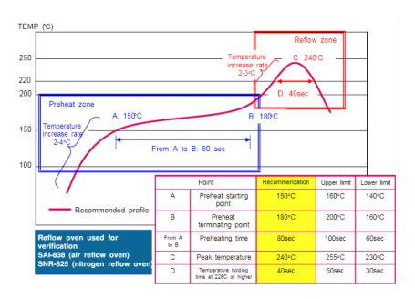
Figure 8-1 Reflow Soldering Profile
