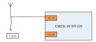
Figure 4-2 UM220-IV NV-GN Active Antenna Solution
