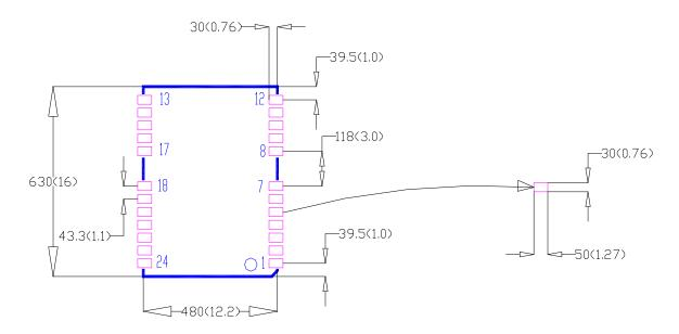
Figure 3-3 UM220-IV NV-GN Recommended PCB Packaging (unit: mil, in brackets: mm)
